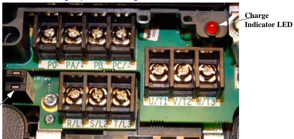
Figure 2. Typical P9 ASD Input/Output Terminals, Charge Indicator LED, and the Grounding Capacitor Switching .
